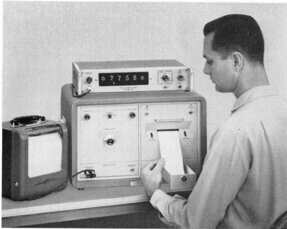
Fig. 1. New -hp- Model 562A Digital Recorder (center) operates from BCD codes to print digital data such as from counters on paper tape. Unit also has option of analog output to drive strip recorders.
